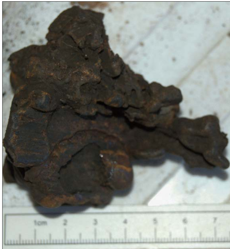
Figure 70. Tap slag from context 048 showing charcoal impression (scale = 7cm).
