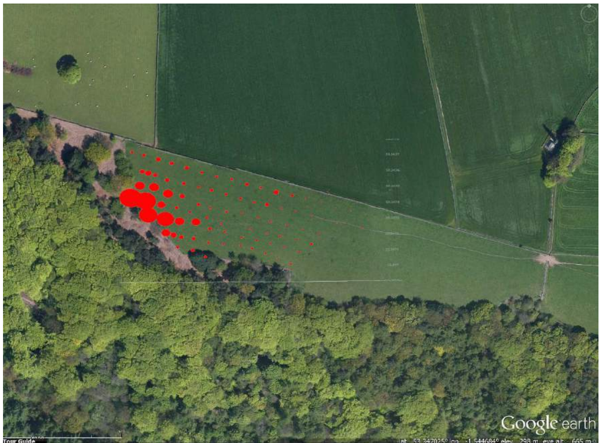
Figure 93. Results of geochemical analysis (Pb) superimposed and georeferenced on Aerial photo.
