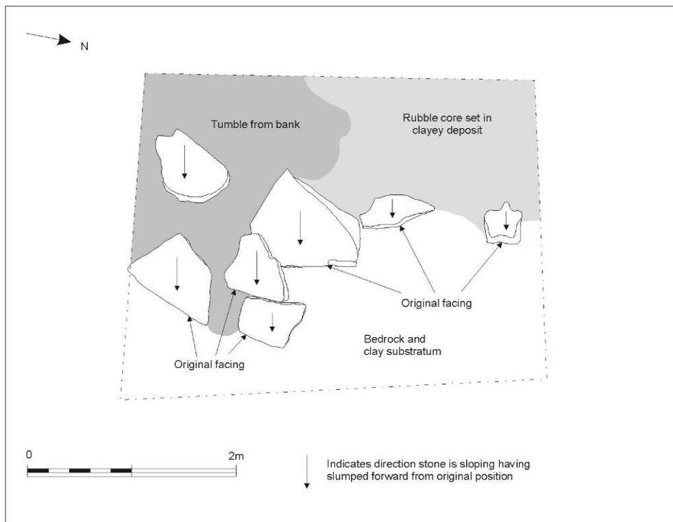
Figure 26. Plan of Trench 4 showing the pitch of the slumped facing stones of the rampart.
