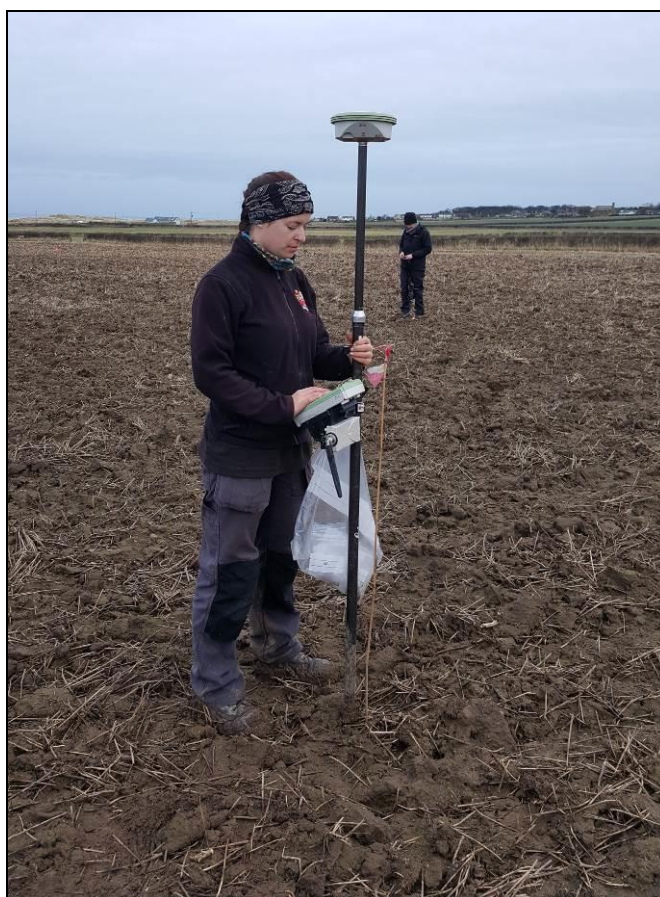
Figure 3. Using the GPS equipment to accurately map the location of each find that had been marked with a cane.
