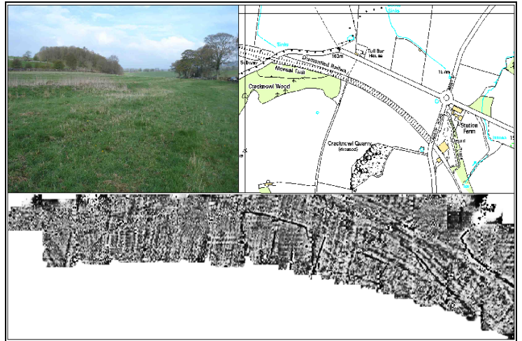
Processed geophysical survey with OS map and photograph of study area
